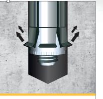
Heavy Duty Self-Undercutting Anchors create a durable mechanical interlock with flooring, giving exceptional pull-out resistance under extreme
