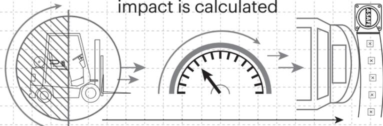
$\frac{1}{2} \text{ Mass} \times \text{Speed}^2 = \text{Joules}$
