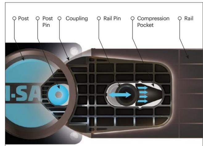
**PHASE 1:** Memaplex™ rail flexes to absorb impact, initiating the rail pin to slide forward and transfer load energy to the compression pocket.
