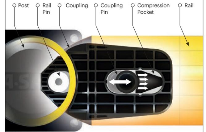
**PHASE 1:** Memaplex™ rail flexes to absorb impact, initiating the rail pin to slide forward and transfer load energy to the compression pocket.
